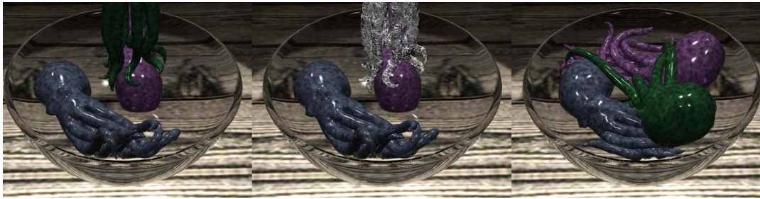
Fig. 9. Octopi Benchmark: Three deforming octopi with 24 tentacles consist of 17.6K tetrahedra. The simulation has multiple inter-object and intra-object collisions. The average CCD query time is 75ms per frame.
