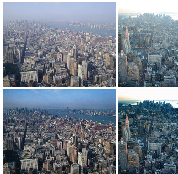
Figure 8: City result. First row: input haze images. Second row: final haze-free image. In this example, \kappa is chosen as 0.5, parameter \lambda is set to 0.01 and t_0 is set to 0.45.
