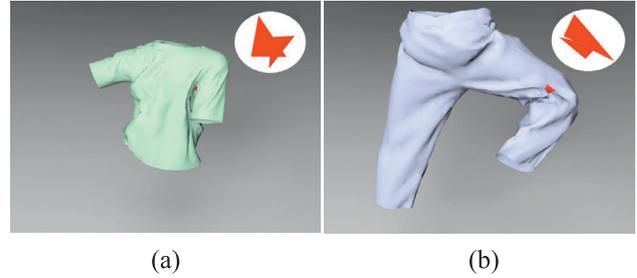
**Fig. 4.** Cloth. For these two cloth simulation benchmarks, the dual-cone method cannot detect the colliding triangle pairs shown in red. (For interpretation of the references to color in this figure legend, the reader is referred to the web version of this article.)
